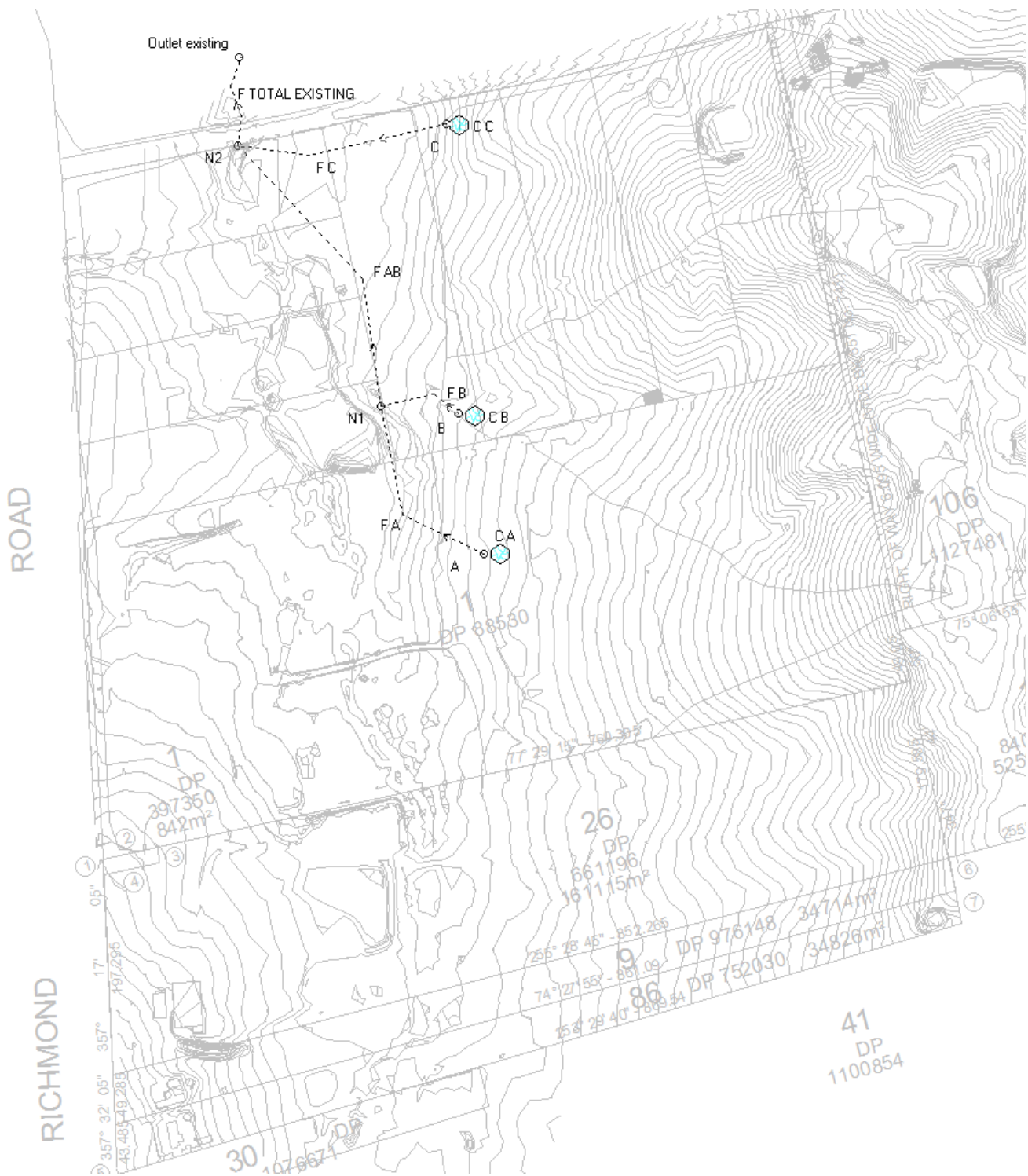
Figure 11 – Existing conditions DRAINS model
