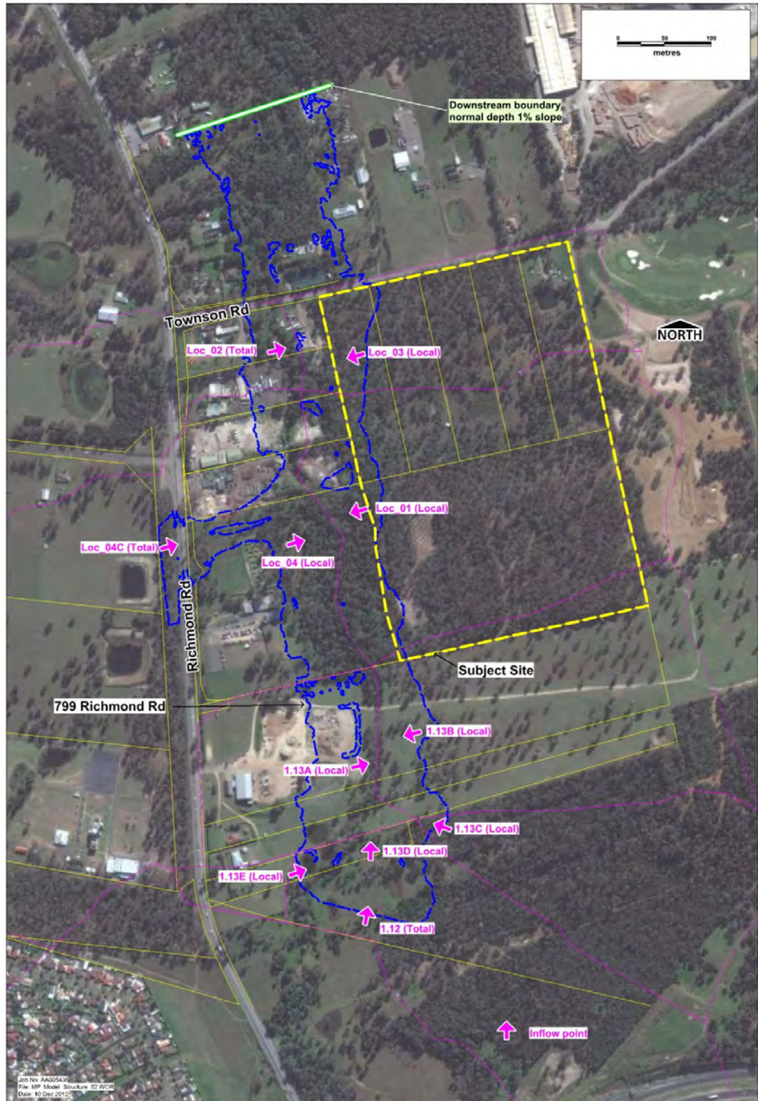
Figure 7 – TUFLOW model structure and flow boundary
